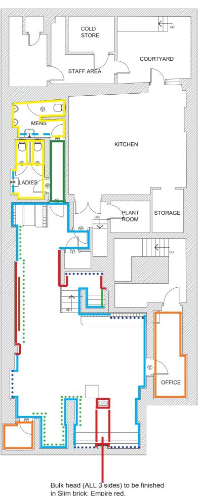
Paint Finish: Dulux 30GY 11/76 Dark Bamboo Cladding Paint Finish: Dulux 60YY 33/130 Paint Finish: Dulux 40YY 67/087 Slim Brick: Empire Red including flat moss Wall covering with Brass Trimming: Vescom, Espalin 2611.02 Lower Wall Panelling: Dulux Heritage Mallard Green (shown on page 28) ••••• Antique Mirror Garden/ Moss Wall with Logo sign to center Horizontal wooden panels (shown on page 29)
